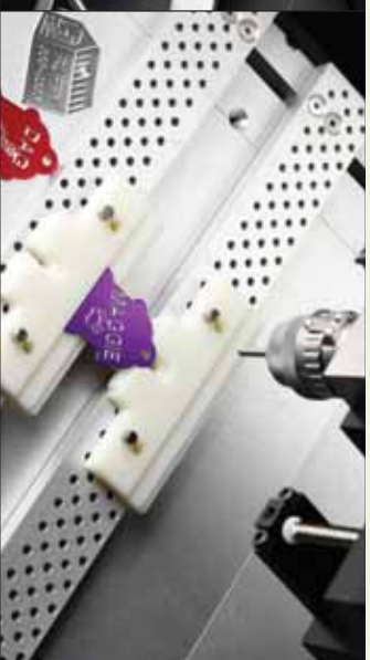
GE self centering vise for engraving small and odd shaped jewelry and gift pieces.
